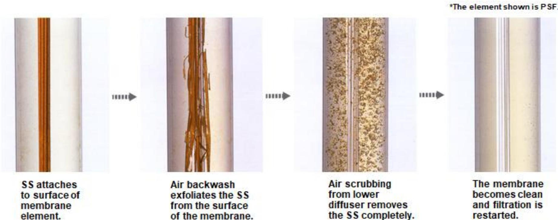
**Air backwash increases water recovery rate — wasted water is only from housing holdup, no permeate is used. No need of permeate tanks or backwash pumps, thus the system is simple and compact and less expensive.**
